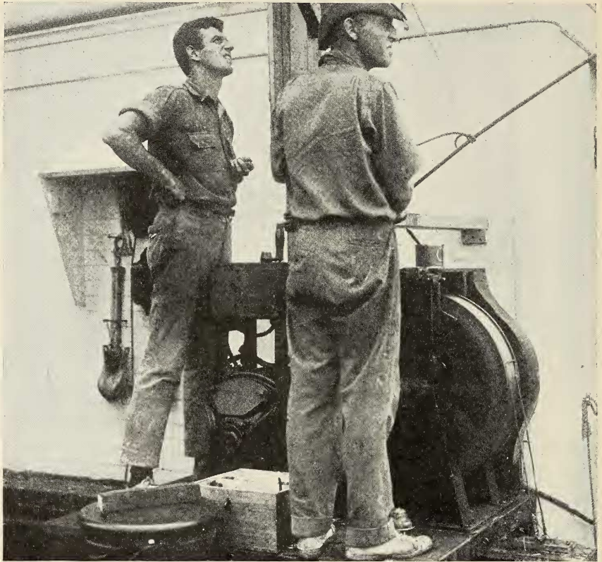
Fig. 8. The sounding machine. To the right is the "tell-tale rod." The controller handle and electric motor are between the two figures.
